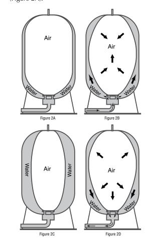
Figure 2: Air Cell Cycle
