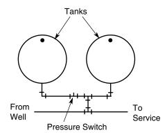
Figure 1A: Typical Layout With Two Tanks
