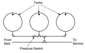
Figure 1B:Typical Layout With Three Tanks
