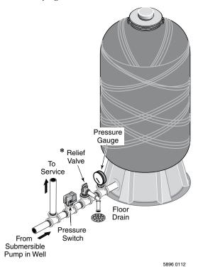
Figure 5: Typical Installation with Submersible Pump
