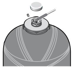
Figure 3: Use A Tire Gauge To Check Pre-charge In Air Cell
