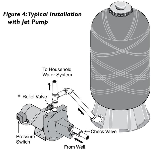
**Figure 4: Typical Installation with Jet Pump**
