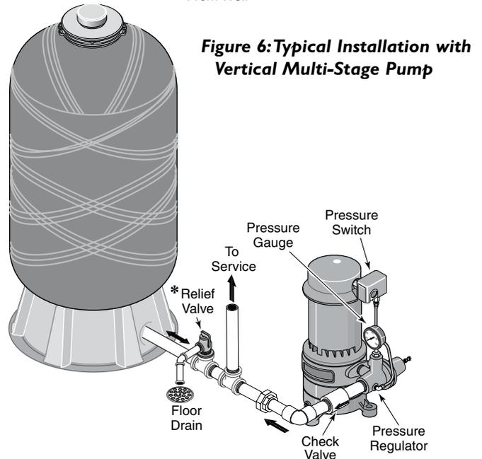
**Figure 6: Typical Installation with Vertical Multi-Stage Pump**
