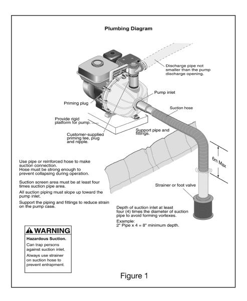
A self priming pump only needs to be manually primed at the first start up. Once primed, under normal conditions the pump will reprime automatically at each subsequent start up. If the pump is used in portable applications and the water has been drained from the pump case, repriming will be required before start up.
